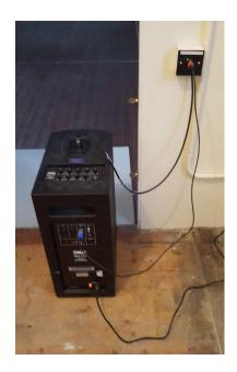
jack plug lead coming from the back of the wall box into the top of the speaker.
